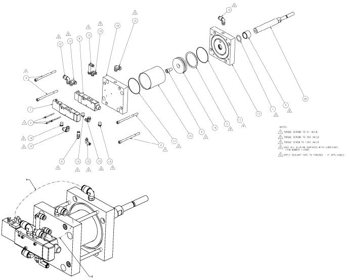
Figure 43: PR70 Air Cylinder Assemblies, 3.0" & 4.5" Diameters (LC0110 & LC0111)
